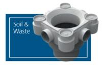
PVCu push-fit and solvent weld systems, ideal for domestic and commercial applications. Innovative fittings include the 8-way collar boss with top and side entries which allow for multiple inlet connections.
